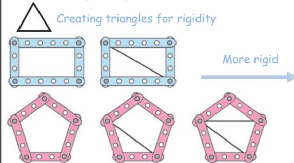
Making small-scale frame structures
